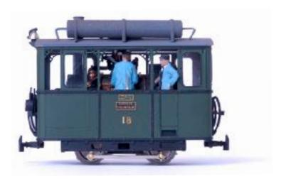
Build date Builder Factory number Water capacity Weight (running) Steam system Maximum speed 1921 Henschel & Sohn, Kassel (D) 18776 2 m3 17 tons Walschaert 45 KM/H
